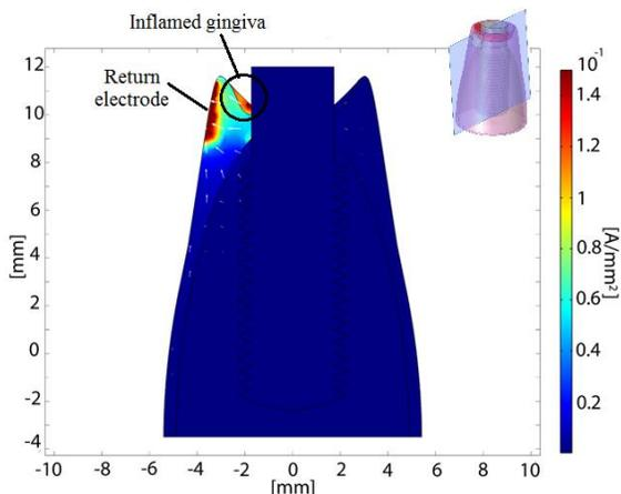
Figure 4: Distribution of electric current (frontal section of the model); apart from edge effects on the electrode, it can be observed that the maximum current density is in correspondence of the inflamed gingiva
