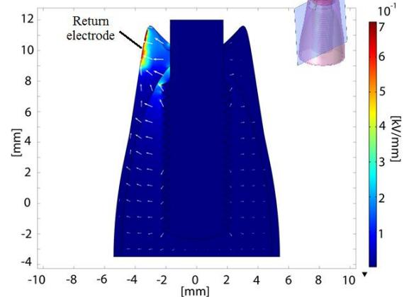
Figure 5: Distribution of electric field lines (frontal section of the model); it can be observed that they significantly involve also hard tissues, on the contrary of the electric current
