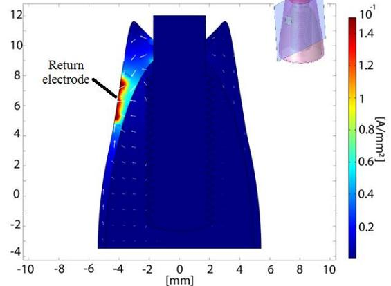
Figure 6: Distribution of electric current (frontal section of the model) in case of return electrode placed lower; it can be noted that current lines are driven by this electrode position
